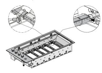
Release the burner from the retaining bracket by lifting as shown.
