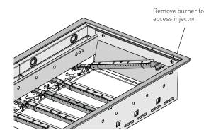
Replace the injector with appropriate size injector (refer to Gas Specification Table on page 6).
