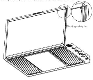
When closing the lid the safety leg will pivot forward and rest against the trim surface to prevent the lid closing.
